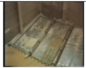
successive layers of product collapse and are gently carried down, until the floor is perfectly clean.
