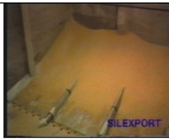
The membrane shaken by high quality Silexport vibrators.
